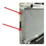
o Gambler filler neck – This filler neck is used on a lot of street rod style radiators. It is used to move the filler neck away from the radiator.
