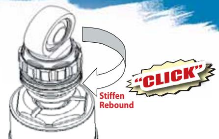
**The compression adjustment** is made on the body end of the shock. Turning the knob clockwise tightens the valving, making the shock stiffer to compress (right hand threads). This adjustment is also commonly referred to as the "Bump".
