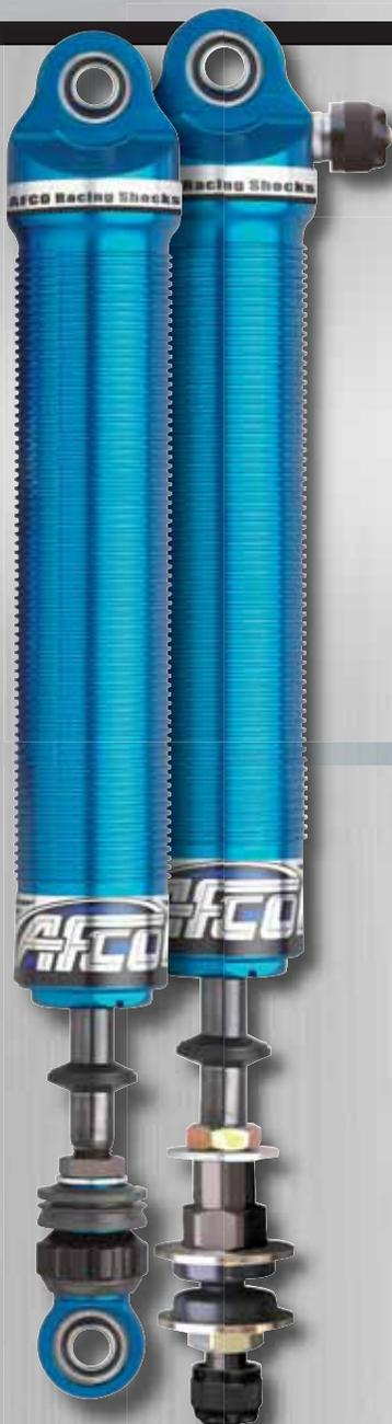
The compression adjustment is made on the body end of the shock. Turning the knob clockwise tightens the valving, making the shock stiffer to compress (right hand threads). This adjustment is also commonly referred to as the "Bump".
