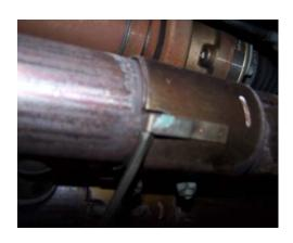
Next remove the catalytic convertors from the manifolds
