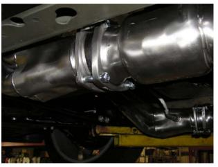
(**On Boss 302 Models**) Connect and snug up the bolts connecting the side pipes to the x-pipe.
