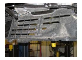
Next unbolt the plastic oil change access cover under the front of the engine. It is made to be loosened in the front and swings down and hangs in place.
