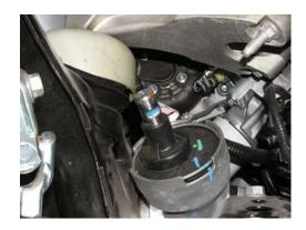
Remove the red plastic cap protecting the starter terminals and disconnect the wiring from the terminals
