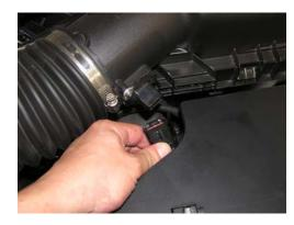
Check all work for completeness, bolts tightened, connectors connected, and lines replaced and clamped etc. Check that no wires or lines are close to the headers where heat damage could occur or near moving parts where they could be pinched or cut. Check for misplaced tools and rags and check for oil leaks etc.
