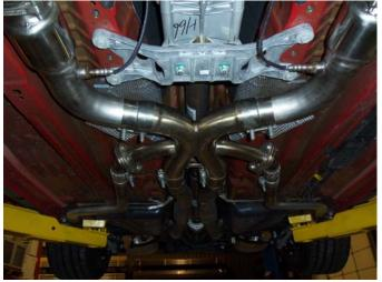
• Start the alignment process at the rear of the vehicle. Twist and align the exhaust outlet to center-up the tip in the body opening. Work your way forward aligning and tightening each of the band clamps to maintain the exhaust tip position in the body opening. Upon reaching the header/catalytic converter joint, tighten the bolts equally to compress the donut gasket slightly to form a leak proof seal.
