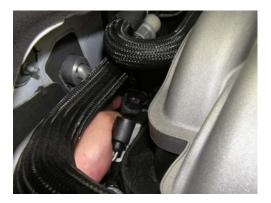
Remove the outside nuts holding the cats to the manifolds on both sides
