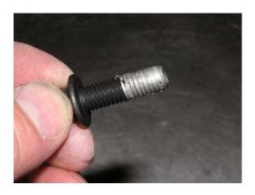
Prepare each of the 16 header bolts with a small amount of antiseize on the thread surfaces.
