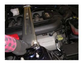
Remove the engine cover (not applicable on the Boss 302)
