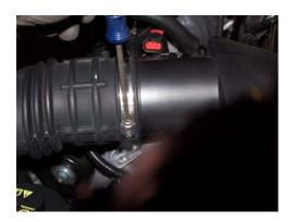
While the vehicle is still on the ground, remove unplug the front O2 sensors located between the rear of the engine and firewall above the transmission bell housing. Install left front O2 sensor extension at this time.
