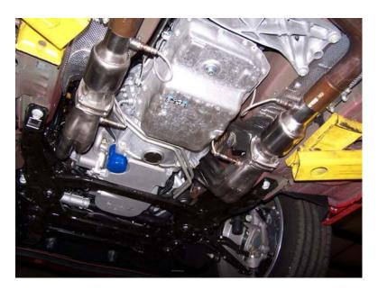
Note: Proper operation of the O2 sensors is crucial for performance and good air-fuel ratio. Please handle with care and keep hands free from contaminating the sensor surface. All sensors should be considered as delicate instruments and should be handled accordingly.
