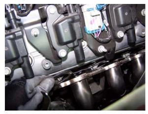
Begin the installation of the rear portion of the system by slipping the 3.0" donut gaskets over the ends of both collectors. Install front 02 sensor extensions.
