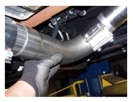
• Install y-pipe outlet extension and bolt to back half of exhaust and band clamp it to the back of the y-pipe. Snug the band clamp but do not fully tighten.
