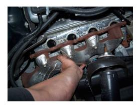
This completes the stock system removal process. Survey the area for stray rags, tools, nuts and bolts, etc. prior to proceeding to <u>"Installing</u> Your New SuperMaXX Header System".
