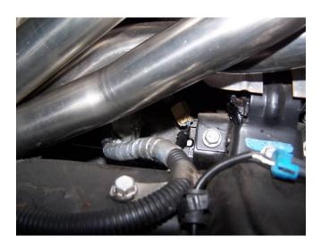
• Retrieve four (4) hex head bolts and top-lock hex nuts from the skin card pack. Put a small amount of anti-seize on each of the bolts. Put the PowerCAT up to the mating surface of the collector and start the nut and bolts through the clamping rings. Equally tighten these nuts and bolts so that the converters are self supporting.
