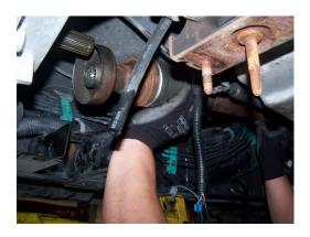
Remove all four (4) of the O2 sensors from the stock exhaust system. Be careful not to ruin the threads during removal. Threads have been known to gall during disassembly. If this occurs, your only choice is to replace any damaged parts with new ones. As each sensor is removed, mark it accordingly so that it may be replaced in the same relative location during reassembly.
