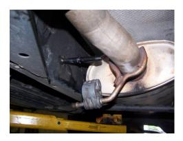
Next, loosen and remove the three (3) nuts on both the left (driver) side and right (passenger) side down tubes and remove y-pipe. Penetrating fluid may be helpful.
