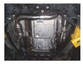
Begin the aligning and tightening process by snugging up all of the clamps and bolts from the collectors back. Each joint or clamp must be free enough to allow for movement during the rest of the process.
