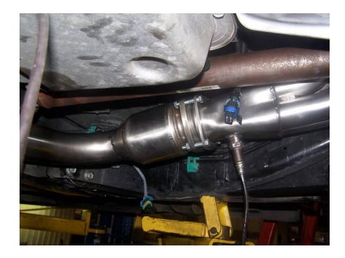
With the cross over tube in place, slip the 2 ½" stainless band clamp over the outlet end of the cross over tube and connect to the y-pipe.
