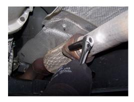
Remove the heat shields from the floor board and the left side frame rail.
