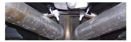
After completing the removal of the cross brace bracket nuts, move forward in the vehicle and remove the four (4) nuts holding the tail pipe assembly to the down tubes. Be careful to support the front end of the tail pipe assembly as the last of the nuts is removed. You may need some help at this point to slip the tail pipe assembly off of the muffler inlet tubes. It is best to do one side at a time until both are removed. The assembly can then be removed from beneath the vehicle.
