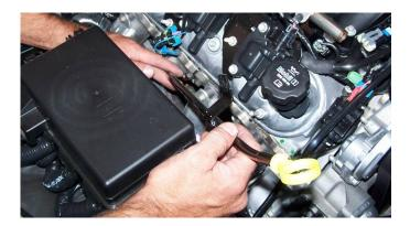
Remove the spark plug wires from both the coil packs and the spark plugs • on both engine banks. (do not pull on the wires, pull on the boots)
