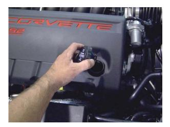
Loosen the bolt holding the oil dip stick tube bracket to the right • (passenger) side engine head and pull the dip stick tube out of the block.
