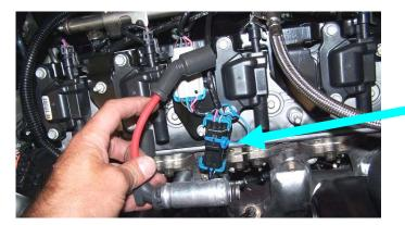
Front O2 sensor connector on the left (driver) side.
