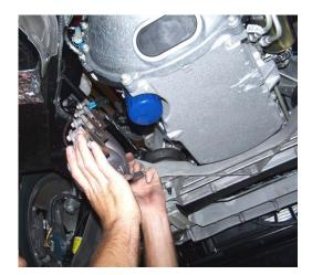
The right (passenger) side cast manifold is removed in a like manner as • the left side. Loosen and remove the six (6) stock manifold bolts and lower the manifold out the bottom of the vehicle.
