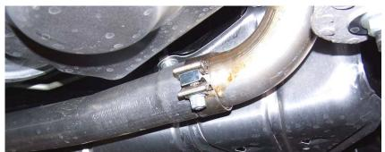
Next, loosen and remove the two (2) nuts holding the stock tail pipe cross brace bracket.
