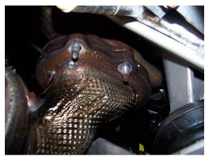
• Once the nuts are removed from the left (driver) side converter assembly, the engine must be raised approximately ½ to ¾ of an inch in order to clear the studs on the bottom of the manifold. Remove the motor mount bolt nut. Then carefully jack the motor up just enough for the assembly to slip off of the bottom manifold studs. Support the converter assembly to prevent damaging the O2 sensors and wiring harness.
