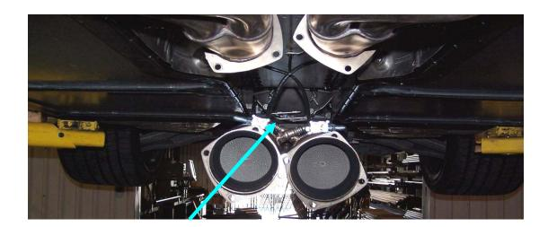
Be sure to attach all the clamps and tie-wraps prior to installing the exhaust system.
