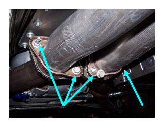
With the bolts and studs removed, lower the front end of the interim tube assembly to the clear the converter tubes. Slide the assembly forward and off of the muffler inlet tubes at the rear. This may take an extra pair of hands and some persuasion with a "dead-blow" mallet. Once the assembly is free from both ends, remove it from beneath the vehicle and store for re-installation should ever decide to go back to the stock system at some point in the future.
