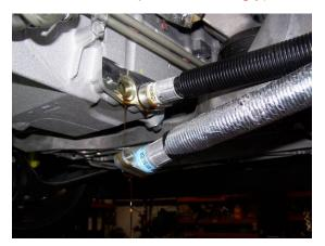
Install the O2 sensor extensions and route them accordingly prior to installing the headers. Clamp and tie them away from any hot or moving surfaces that could cause damage to either the extensions or the sensors.
