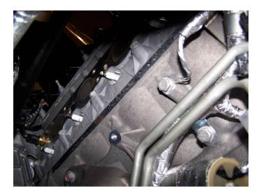
Likewise loosen and remove the six (6) bolts holding the stock manifold from the right (passenger) side of the engine. Once again either remove the sparkplugs or use extra care not to damage them during the removal process. The oil sump lines may have to be flexed slightly to enable the removal of the manifold out the bottom of the engine bay. The engine bay should look similar to the picture below.
