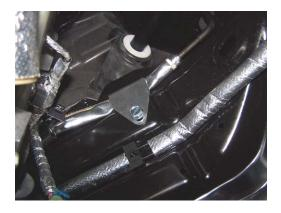
Install the clamp so that the curved part cradles the clutch line and clamps it loosely to the firewall.
