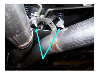
Move forward in the vehicle and loosen and remove the two (2) bolts and the two (2) studs holding the interim tube assembly to the back of the catalytic converter/tube assembly.
