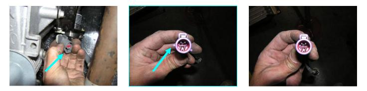
Notice the connectors with the external tabs removed to allow for plug in.
