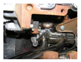
• Locate two of the O2 sensor extension cables. Use these extensions to plug into the front and rear O2 sensor connectors on the left (driver) side in the vehicle wiring harness.
