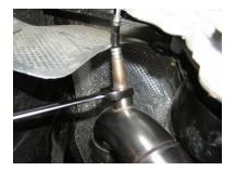
With all of the sensors installed and tightened, connect the sensor connectors into the appropriate extension cable or wiring harness connector as is the case with the right (passenger) side front sensor. (Note: The external tabs on the O2 sensor cables may have to be removed to plug in correctly. See the notes on page 12 of this manual for further information.)
