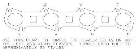
• As in the bolt preparation step above, prepare the eight (8) bolts for the right (passenger) side header with anti-seize.
