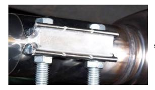
Tighten these clamps very tightly. They work by stretching the metal around the tube preventing any leaks.
