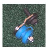
Note: Use a 1/4" drill bit for the "body bolt" used to attach the offset tab to the frame or floor pan. This bolt extrudes the metal, forming a thread that is thicker than the metal thickness itself. Start the bolt, and then finish with a ratchet and socket or an impact wrench and socket. Be careful not to strip the threads out of the sheet metal.
