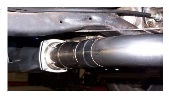
the vehicle. Once you are satisfied that the system is correctly aligned and tightened, start the engine and check for leaks. If any are found, retighten the fasteners around the clamp at issue. All fasteners should be rechecked after the system has gone through several thermal cycles.
