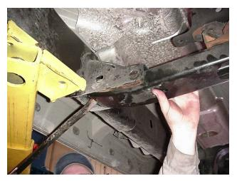
Pry the passenger side of the cross member down to aid in its removal.
