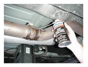
11. Loosen the muffler/"Y"-pipe clamp and separate the muffler from the "Y"-pipe. You may need a dead blow hammer or a rubber mallet to accomplish this. Completely removing the muffler and tailpipe is not required but may help to eliminate interference while removing and installing your new header system.
