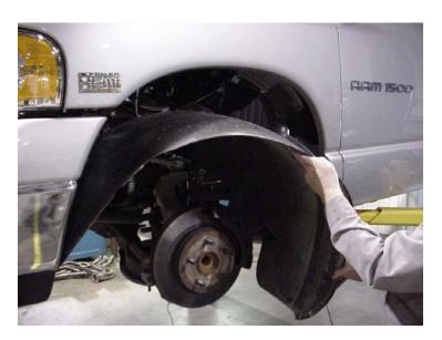
Install panels and screws in the same manner in which they were removed.
