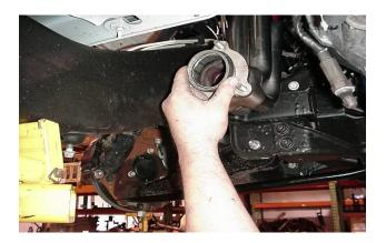
Install the sintered metal donut gaskets before you install the "Y"-pipe.
