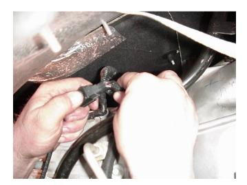
Removal of the actual sensors from the old exhaust system is best performed after the exhaust system has bee completely removed.
