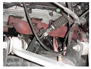
Remove the bolts and heat shield for access to the exhaust manifold bolts.
