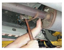
Page 6 of 15 2.doc2 12. Loosen the nuts holding the "down tubes" to the cast manifolds.
