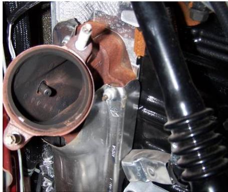
The nuts are fairly easy to remove but will require some effort. The removal of the heat shields is probably the most difficult part of the whole removal process. You may have to bend, twist, and pull just to remove them, but they will come out.
