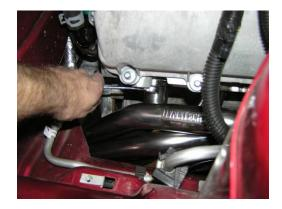
With the engine still supported and slightly elevated, guide the steering intermediate shaft into the universal joint and bump the rack and pinion back into position.
