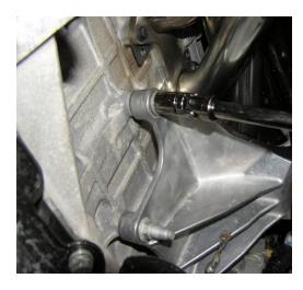
Install the right (passenger side) motor mount by slipping the mount over the stud at the right frame rail and sliding the mount into position on the engine block. Apply a small amount of anti-seize to the motor mount bolts/studs. The studs go in the upper front hole and the lower rear hole. With all fasteners installed into the block, tighten to approximately 40 ft/lbs.
