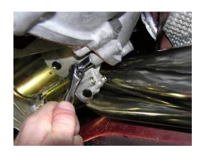
Re-install the starter (three bolts), attach the starter cables, and replace the protective red terminal cap.
