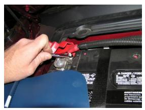
Removal of the battery and tray provides more room to get to the manifold bolts during a later step. Remove the battery cover and tie-down, the
