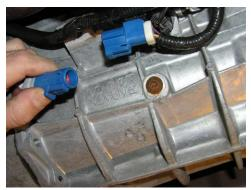
Loosen and remove the 2 rear O2 sensors from the "H"-pipe. Be sure to mark the sensors so that can be put back in the same relative positions in the new system. The front right (passenger side) O2 sensor will have to be removed after the "H"-pipe is removed from the vehicle.
