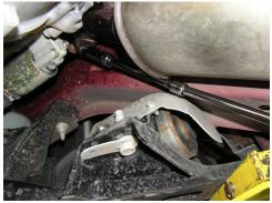
Remove the rear tailpipe couplers that were loosened in an earlier step by inserting the flat of a screwdriver under the spring tab and twisting to release while sliding the couplers rearward. Be sure to save these couplers, they will be reused during the installation of the new system.
