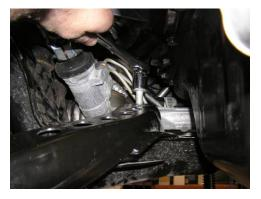
Remove the 2 bolts holding the steering rack and pinion into cross-member.
