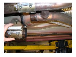
• The "H"-pipe assembly should be completely free to remove at this point. Do this by lowering the rear of the unit and sliding the entire assembly rearward out of the rubber hanger brackets. Lower the rear of the unit to the ground.
