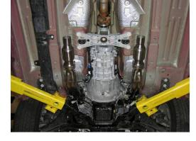
Assemble the "X"-pipe by slipping a band clamp over short leg of the X-pipe and inserting the left interim leg into the clamp. With x-pipe unit assembled slide a band clamp on each of the 2 inlet legs of the x-pipe and slide the whole assembly into the rubber hanger brackets and into the rear of both the left and right catalytic converters. Bend X-pipe hangers to aid alignment if needed.
