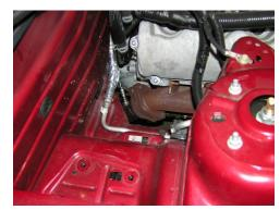
In addition, this is best time to gain access to the nuts that hold the motor mounts to vehicle frame.
