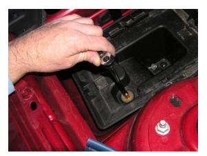
Slide the red retainer clip out on the MAF (Mass Air Flow) sensor and disconnect the harness.
