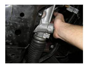
Reinstall the 2 rack and pinion bolts and torque to approximately 45 ft/lbs. Reattach the power steering line clamp in the front cross-member.
