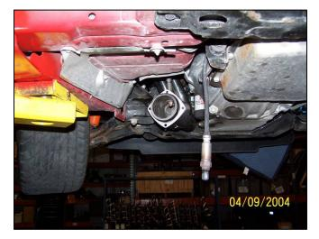
Page 9 of 13 LIT 994 Dynatech Headers, P.O. Box 548, Boonville, IN 800-848-5850 www.dynatechheaders.com Cop yright 2009 AFAB LLC • Slide a 3.0" donut gasket over the end of each collector making sure the flat side of the donut is pushed up tight against the collector stop ring.
