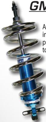
AFCO Racing Products is proud to offer a bolt-in coil over shock system for drag racing. This system allows for bolt-in, no modification installation on most popular GM applications. Some of the features include: easy ride height adjustment, quick corner weight tuning and pre-load changes to straighten out bad launches, and front end weight reduction. From street and strip to all out drag racing, rely on AFCO to deliver two quality suspension components.
